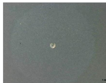
**Fig. 2:** Brightening and pitting corrosion on test piece made of stainless steel X20Cr13 with bead blasted surface after 72 h interaction with mixture from cleaner 2 and blood in ten-times magnification
