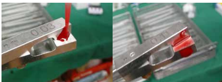
Fig. 2: Contamination of PCDs: pipetting to surface and movement
