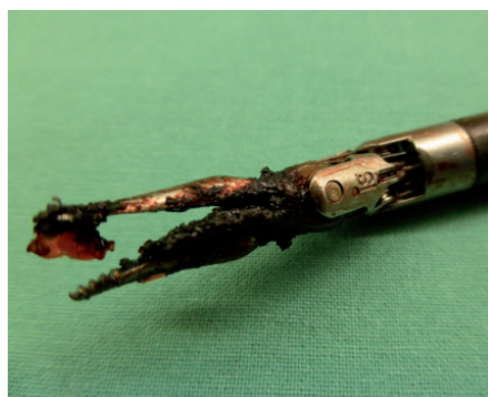
Fig. 3: Cauterization residues on functional end of curved bipolar dissector
