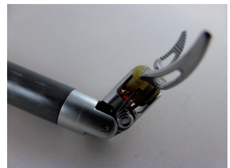
Fig. 2: Visible blood residue on Maryland bipolar forceps of test run 2
